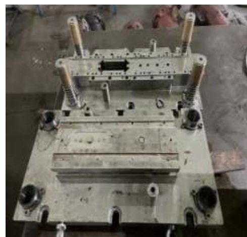
Press Tool for Pressure plate of Ammunition box H60 for Ordnance Factory Bhusawal.
