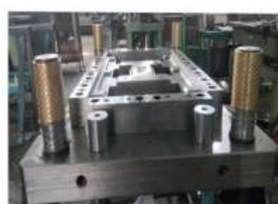
Press Tool Developed for Lid of Ammunition Box for Ordnance Factory
