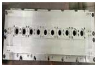
Design & Manufacturing of 10 cavity blow mould for 500ml bottle for Pharmaceutical Industry, Previously it was imported from Germany & Italy.
